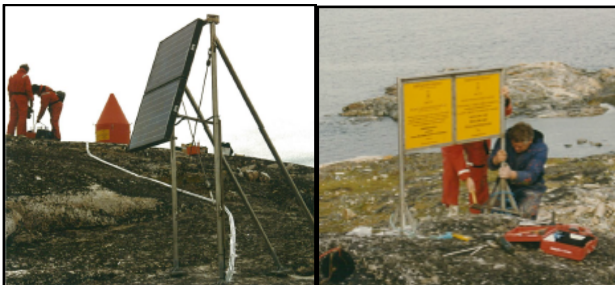
Figure 7 Example of cable protection against wild animals & notices to deter vandalism
